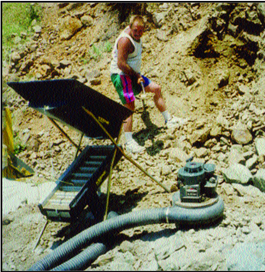
Operating a Vibrostatic Concentrator (Dry Washer) with Hot Air Induction in a dry area of Los Angeles County
