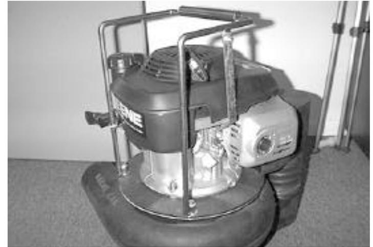
The Honda engine mounts similar to the Briggs and Stratton engine. The Honda requires two extra supports.
