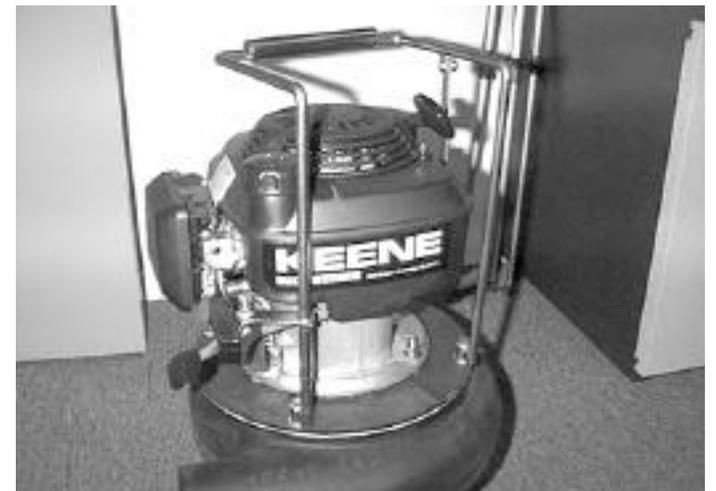
The engine does not come with oil in the crank case. Be sure to add oil.
