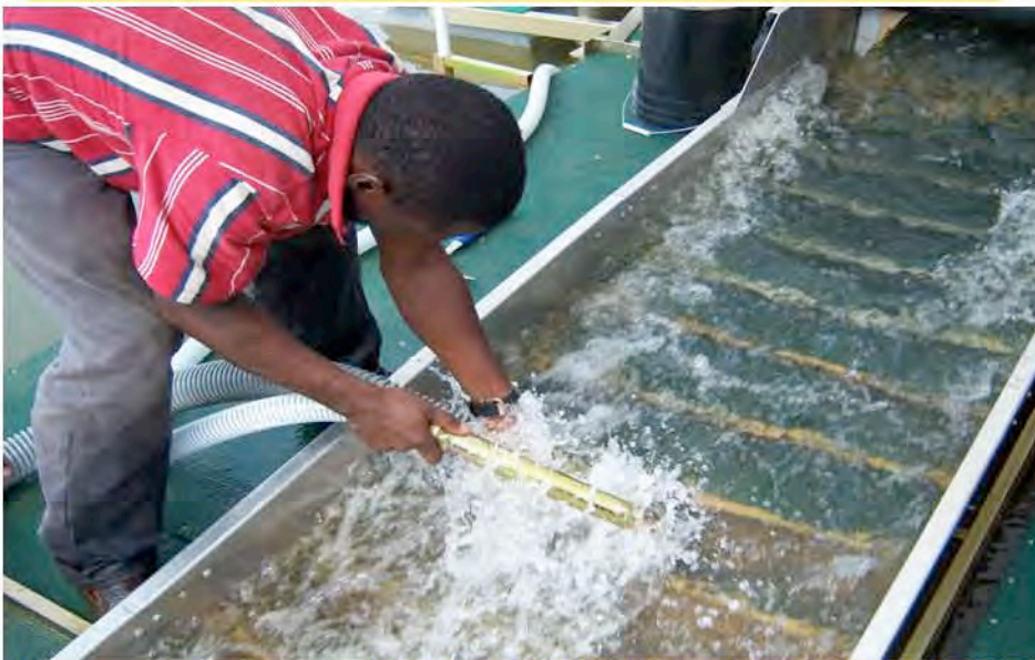
Vacuuming concentrates from main sluice box and filling a rice bag for transportation to shore for final recovery
