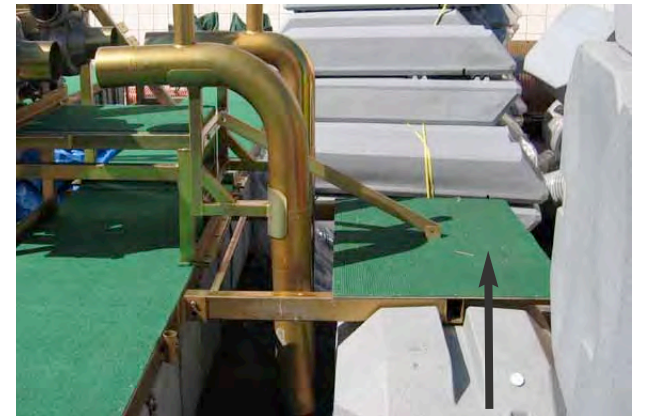
FIG 1F install outrigger side support assembly mount on opposite side of dredge.
