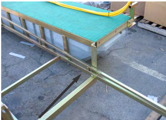
FIG 1G Assemble sluice box ladder to frame and bolts to fig.1C rear sluice box frame support.
