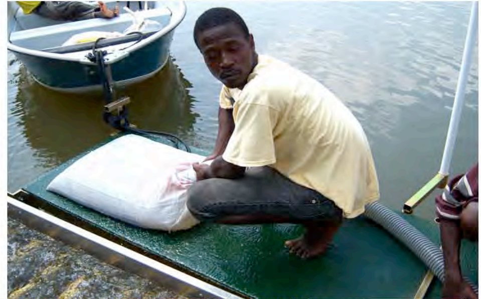
Vacuuming concentrates from main sluice box and filling a rice bag for transportation to shore for final recovery
