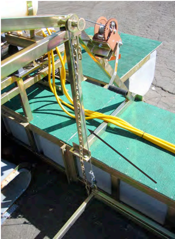
FIG 1J Winch and safety chain is used to raise and lower sluice box assembly.
