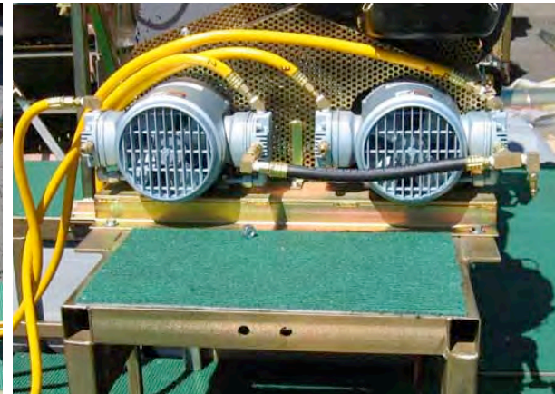
FIG 2C Typical Air Snorkel attachmet to air compressors and air pressure hose assembly
