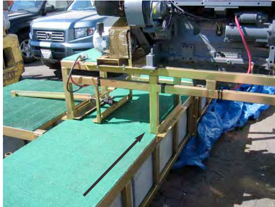
FIG 1K Install engine to mounting brackets on frame deck.
