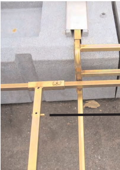
THE ALUMINUM LIP ON THE BOTTOM OF THE SLUICE BOX SLIDES OVER PINS AND IS LOCKED IN PLACE WITH COTTER PINS
